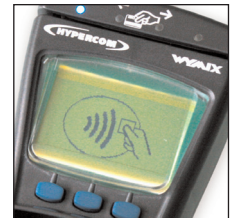
Backlit graphics display with embedded contactless antenna
